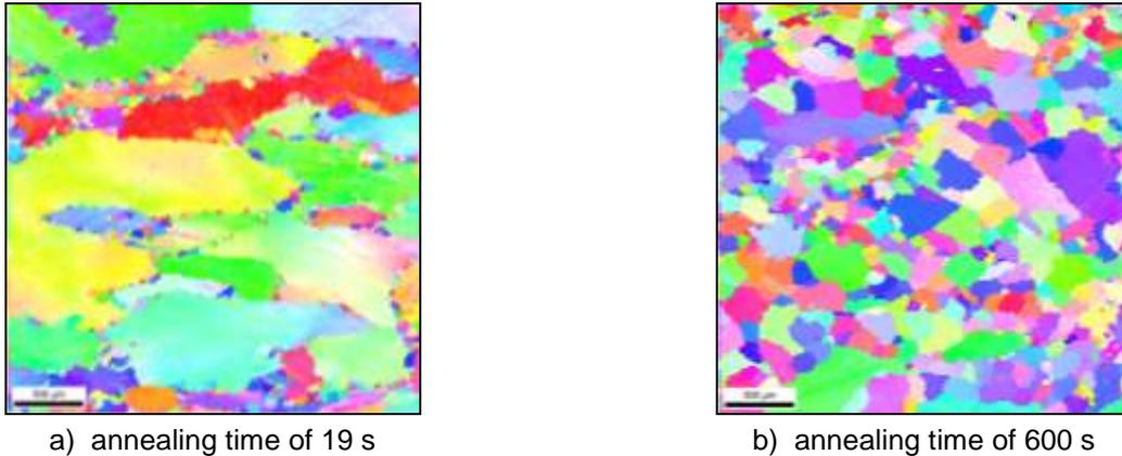
**Fig. 9** Microstructure of the samples annealed at the temperature of 900 °C (EBSD)
