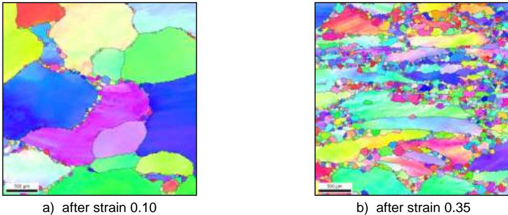
**Fig. 4** Microstructure of the samples annealed at the temperature of 900 °C after different deformation (EBSD)
