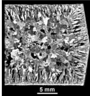
**Fig. 1** Heterogeneous macrostructure of the initial casting (partial cross section)
