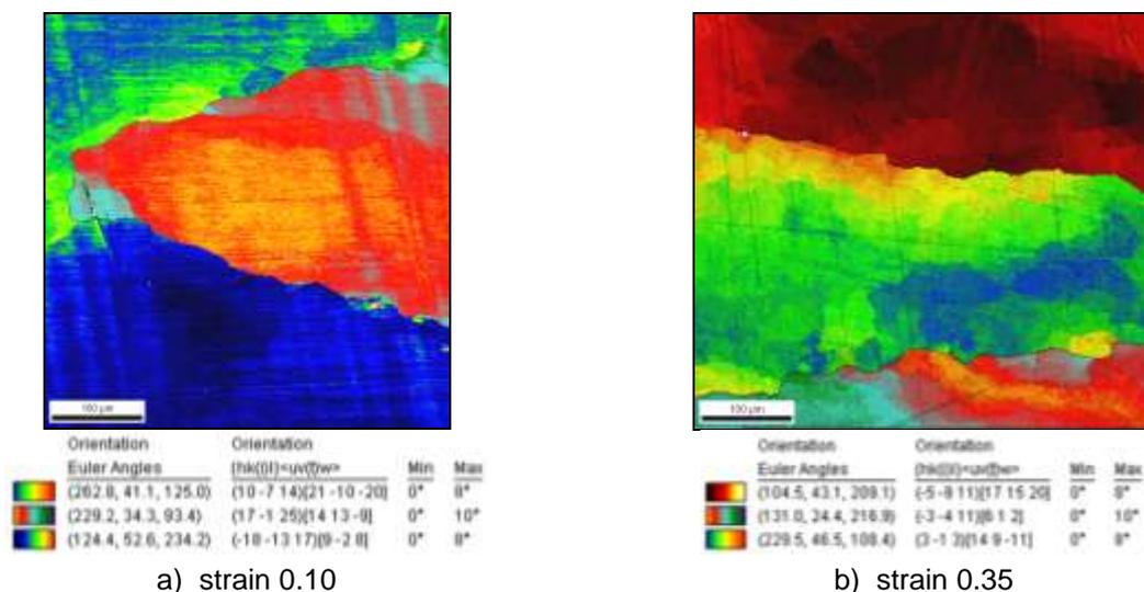
**Fig. 6** Detection of the small angle grain boundaries after annealing at 1100 °C (EBSD+FSD)
