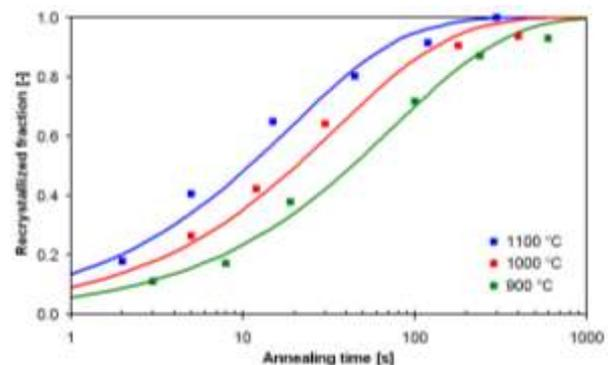
**Fig. 10** Demonstration of the accuracy of Eq. (2) (solid lines) in comparison with experimental data (points)
