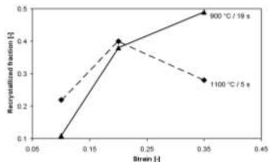
**Fig. 3** Influence of previous deformation on the static recrystallization kinetics
