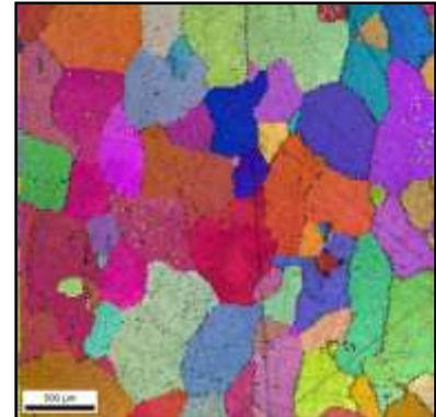
**Fig. 2** Microstructure after homogenization annealing at 1273 °C for 7 hours (EBSD)
