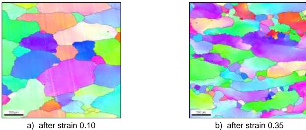
**Fig. 5** Grain size maps of the samples annealed at temperature 1100 °C (EBSD)
